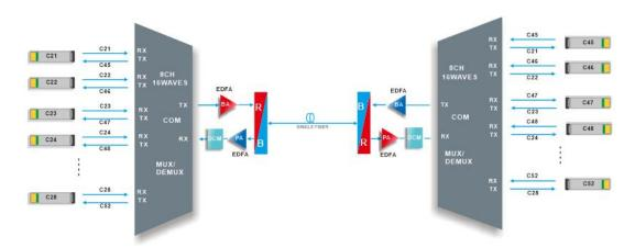
8CH DWDM MUX/ DEMUX Single fiber transmission
