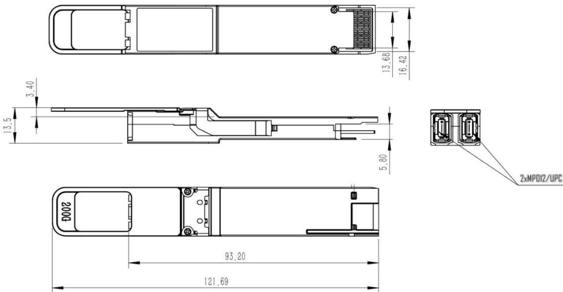
Figure 3 – Mechanical Dimensions for 2\*MPO12
