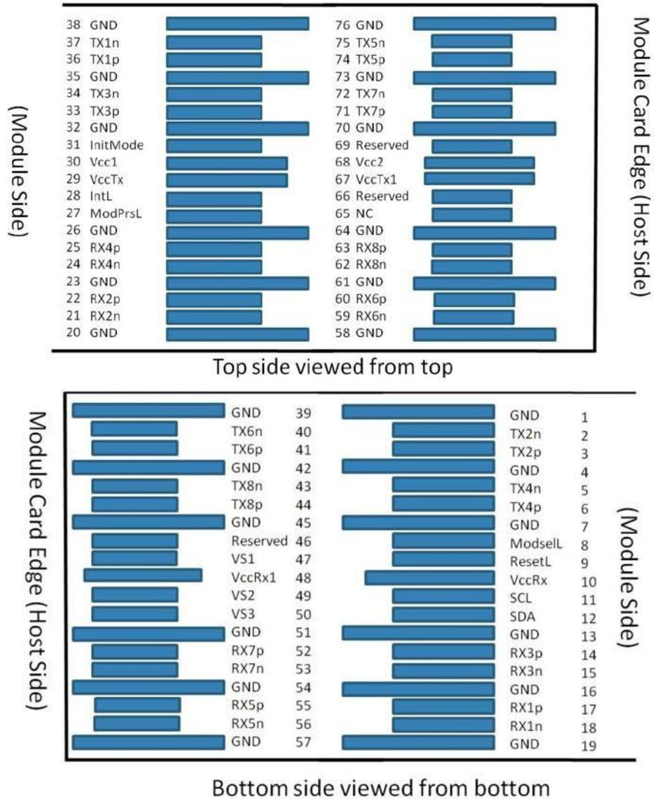
Figure 1 –Module Pad Layout
