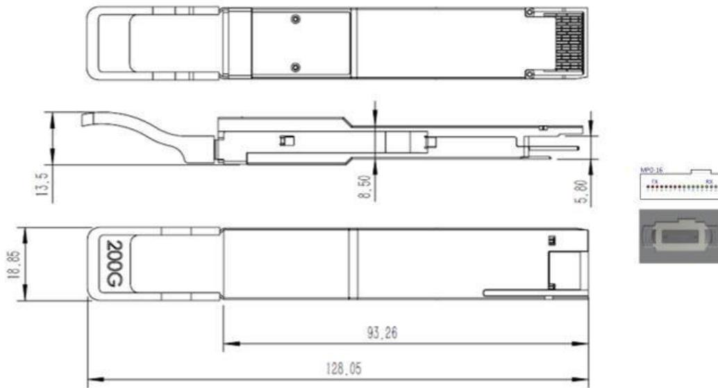
Figure 2 – Mechanical Dimensions for MPO16
